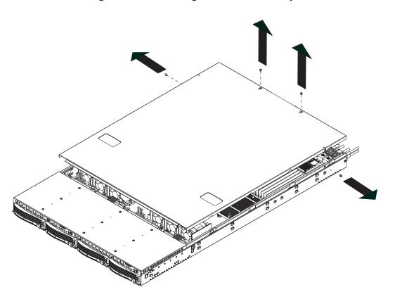
Figure 2-4. Accessing the Inside of the System
